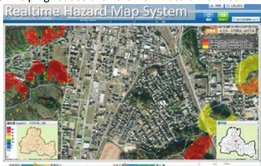
Fig.1 Our Realtime Hazard Map reflects up-to-date information of soil natures and precipitations at landslide hazard sites, etc. that can constantly be changing, and evaluates area-wide hazard risk in real-time
